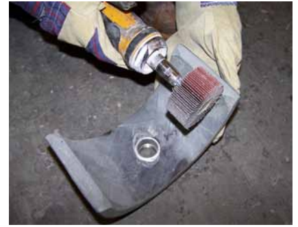
Sand the inside surface of the saddle
