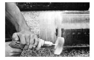
• Buff up the interior of the bell and remove any rough edges using a flapper sander or sandpaper.
